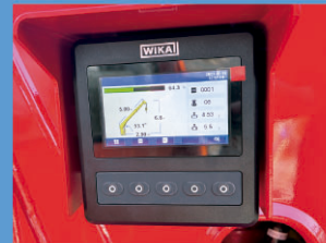
Safe Load Indicator
