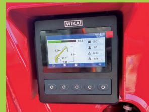
Safe Load Indicator
